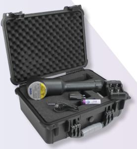
UniVario is also compatible with the **UniVario FLS-1 Ex Flame Simulator**, ensuring reliable testing of IR flame detectors. Designed to work at distances of up to 9 meters, this flame simulator simplifies commissioning, diagnostics and maintenance, saving you time and avoiding costly interruptions.
