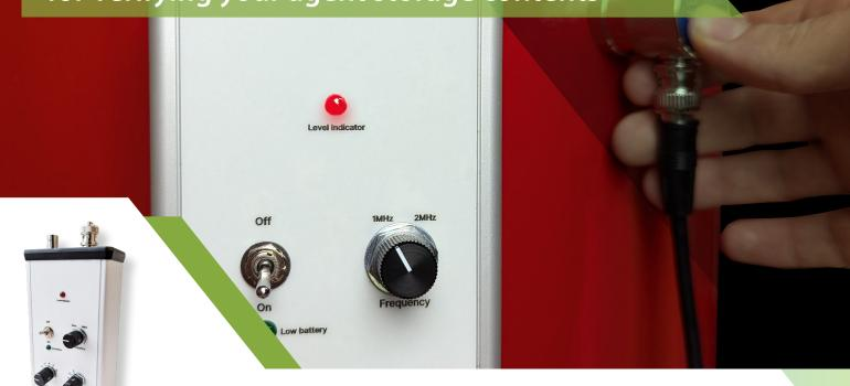
The ultrasonic liquid level indicator (ULLI) is a compact, easy-touse tool designed to quickly measure the agent content in gas cylinders. In just seconds, you can verify the liquid level by placing the ultrasonic sensor on the cylinder. An LED lights up precisely under and at the liquid level, providing a clear and reliable indication without the need to dismantle the cylinder or to call an expert.
